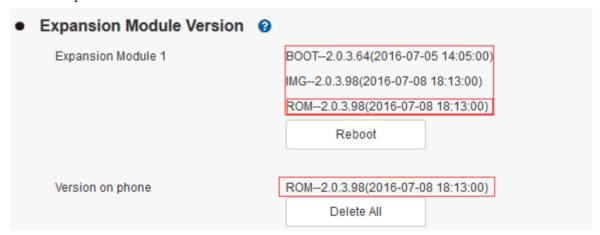
(5) If expansion module FW did not upgrade successfully, please restart the expansion module to upgrade the FW again.
